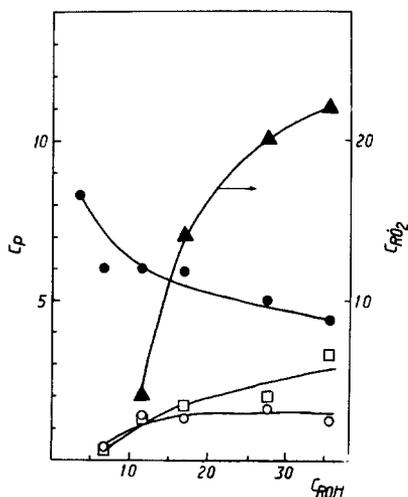
FIG. 5. Effect of alcohol concentration in initial mixture on accumulation of radicals ( $C_{\text{RO}_2} \times 10^{11} \text{ ml}^{-1}$ ) and stable products ( $C_p$ , vol.%) in oxidation of *n*-propanol over Pt/ $\gamma$ - $\text{Al}_2\text{O}_3$ ,  $C_{\text{O}_2} = 15.0$  vol.%,  $T = 823$  K. ( $\square$ )  $\text{CH}_3\text{CH}_2\text{CHO}$ , ( $\circ$ )  $\text{CH}_2=\text{CHCH}_3$ , ( $\bullet$ )  $\text{CO}_2$ , ( $\blacktriangle$ )  $\text{RO}_2$ .
