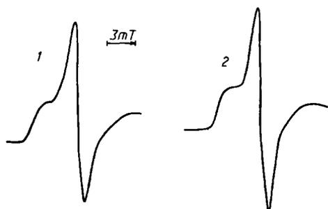
FIG. 2. ESR spectra of radical frozen out from gas phase at 77 K after oxidation of *n*-propanol over  $\text{CuCr}_2\text{O}_4/\gamma\text{-Al}_2\text{O}_3$  (1) and  $\text{Pt}/\gamma\text{-Al}_2\text{O}_3$  (2).
