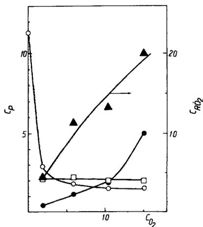
FIG. 4. Effect of oxygen concentration in initial mixture on accumulation radicals ( $C_{RO_2} \times 10^{11} \text{ ml}^{-1}$ ) and stable products ( $C_p$ , vol.%) in oxidation of *n*-propanol over Pt/ $\gamma$ -Al<sub>2</sub>O<sub>3</sub>,  $C_{ROH} = 27.6$  vol.%,  $T = 823$  K. (□) CH<sub>3</sub>CH<sub>2</sub>CHO, (○) CH<sub>2</sub>=CHCH<sub>3</sub>, (●) CO<sub>2</sub>, (▲) RO<sub>2</sub>.
