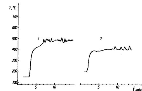
FIG. 6. Periodic changes of catalyst temperature in oxidation of *n*-propanol (11.2 vol.%) by stoichiometric amount of oxygen (50.7 vol.%) over catalysts: (1) Pt/ $\gamma$ - $\text{Al}_2\text{O}_3$ , (2)  $\text{CuCr}_2\text{O}_4/\gamma$ - $\text{Al}_2\text{O}_3$ .
